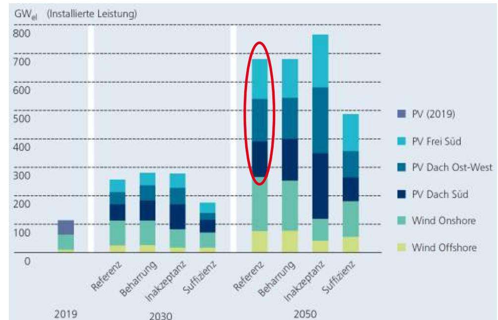
Cumulative installed capacity of PV and wind power for four examined scenarios, Fraunhofer ISE
