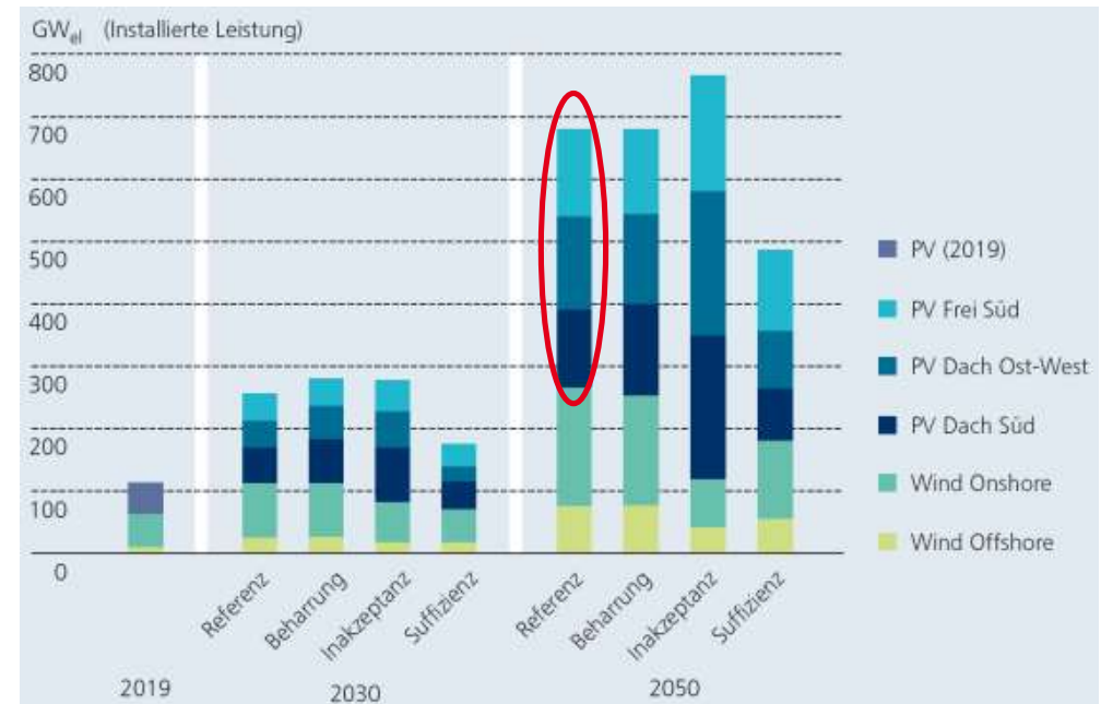
Cumulative installed capacity of PV and wind power for four examined scenarios, Fraunhofer ISE Febr. 2020
